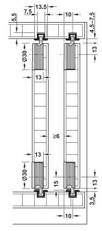
(A) Guide with lockable bolt C Running gear with height adjustment
